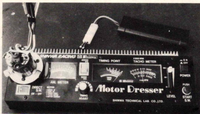
This photo shows the Motor Dresser with the motor timing having been set to 0 degrees, in accordance with the unit's instructions. Full revs are not required for this operation, as indicated in the text.
